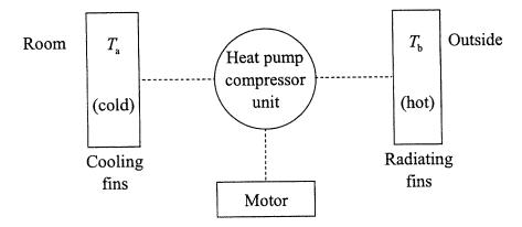
(a) The dotted lines in the diagram show routes of possible energy flow. Complete the diagram by drawing in labelled arrows representing the energy flows (both heat and work). Use thicker arrows for greater energy flows.
