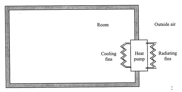
A schematic diagram of the heat pump and heat transfer fins is shown below.
